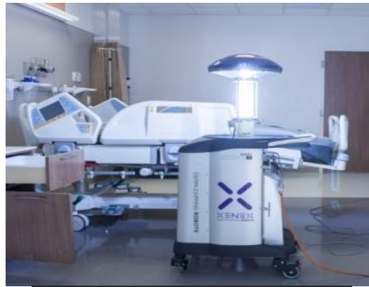
UVGI unit indoor
