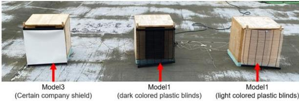
Fig. 2 Model experiment of model 1 (light colored plastic blinds), model 2 (dark colored plastic blinds) and model 3 (Certain company shield)
