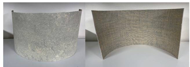
Fig.2 Flooring sheet made of linoleum
