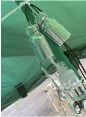
Fig.4 Thermocouple with radiation shields
