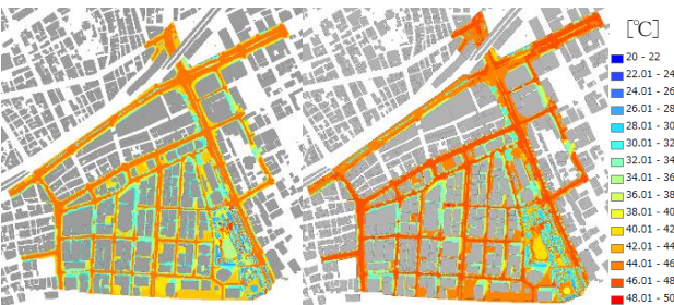
Fig.7 Distribution of surface temperature (left) and MRT (right) at 13:00 on August 5, 2019
