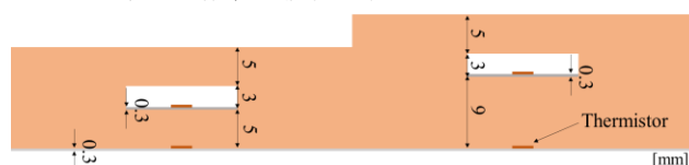
Fig.17 Cross section of insulation.
