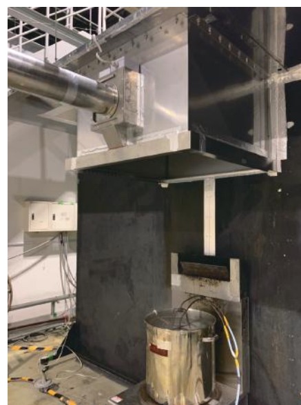
Fig.2 Exhaust Hood equipped with Additional Jet Device
