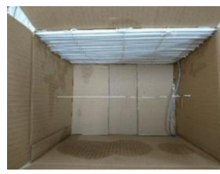
Fig. 2 Installation status of PCM bamboo blind
