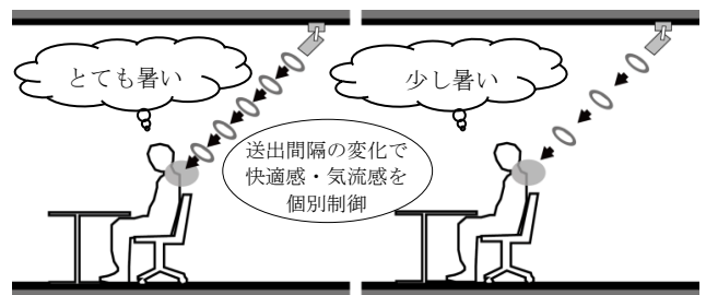
Fig. 1 Pulse airflow diagram
