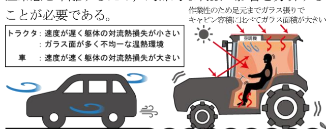
Fig.1 Difference of Thermal Characteristic Between Car and Tractor Cab
