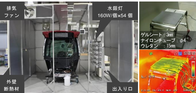
Fig.3 Views of the Laboratory and Cooling Chair, Thermal Image
