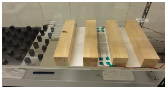
Fig.1 Arrangement of model and surface heating element (in the wind tunnel)
