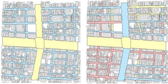
Fig.4 Weak wind risk distribution based on street width (left) and CFD analysis result (right)
