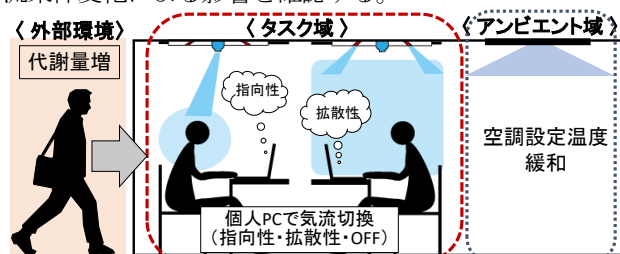
Fig.1 Personal Air-Conditioning System with selectable Air Flow
