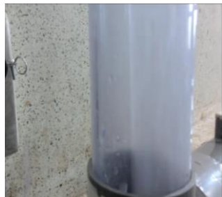
Figure 4 Transparent piping in the conditions of the drainage flow rate 0.3L/s
