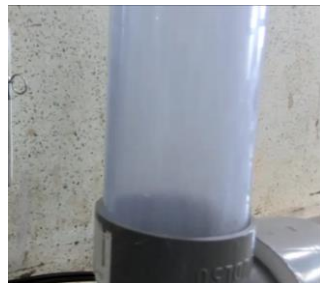
Figure 3 Transparent piping in the conditions of the drainage flow rate 0.4L/s
