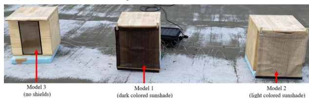
Fig. 12 Model experiment of model 1 (dark colored sunshade), model 2 (light colored sunshade), and model 3 (no shield)
