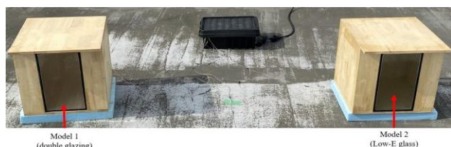
Fig. 2 Model experiment of model 1 (double glazing) and model 2 (Low-E glass)
