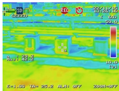
Fig. 14 Thermal cameras of model 1 (dark colored sunshade), model 2 (light colored sunshade), and model 3 (no shield) at 13:26 on November 15, 2022
