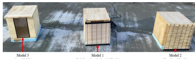
Fig. 4 Model experiment of model 1 (bright colored plastic blinds), model 2 (bamboo blinds), and model 3 (no shields)
