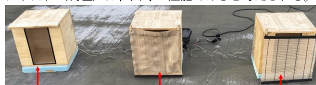
Fig. 10 Model experiment of model 1 (light colored sunshade), model 2 (light colored plastic blinds), and model 3 (no shield)
