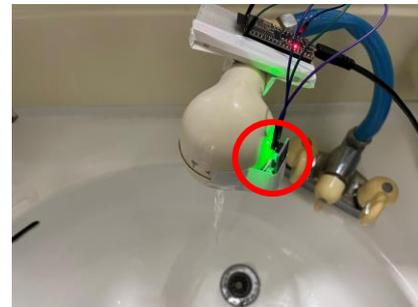
Fig.14 Sound sensor installed at the tip of the spout (home)
