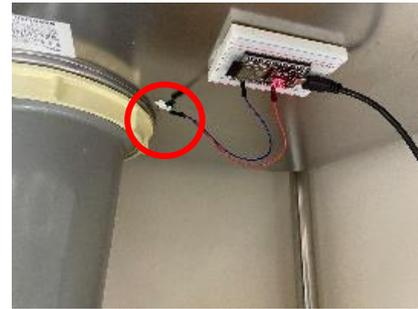
Fig.5 Vibration sensor installed on the back of the sink (lab)
