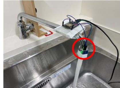
Fig.12 Sound sensor installed at the tip of the spout (lab)
