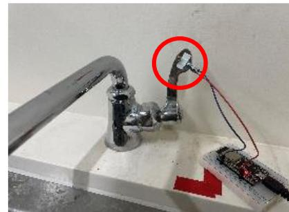
Fig.8 Vibration sensor installed on lever handle (lab)
