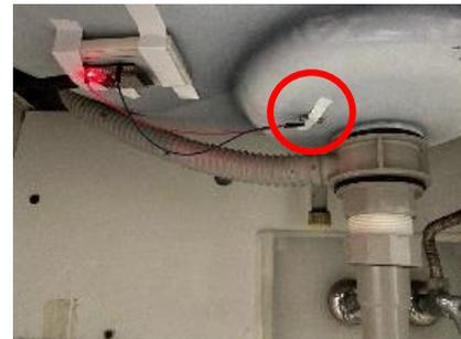
Fig.7 Vibration sensor installed on the back of the sink (home)
