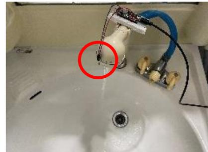
Fig.6 Vibration sensor installed at the tip of the spout (home)
