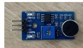
Fig.3 VKLSVAN Sound Sensor Module
